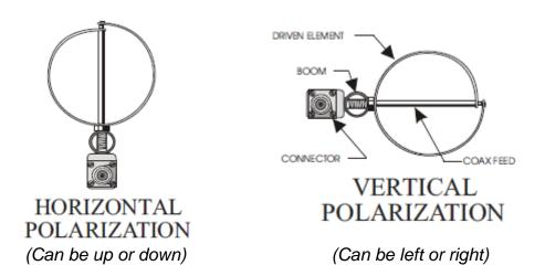
5) Attach the feed line, and tape it to the mast. The connector should be sealed with electronic grade RTV or equivalent.
