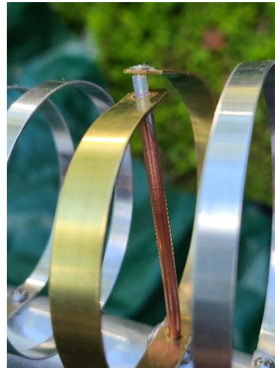
Soldered Driven Element
