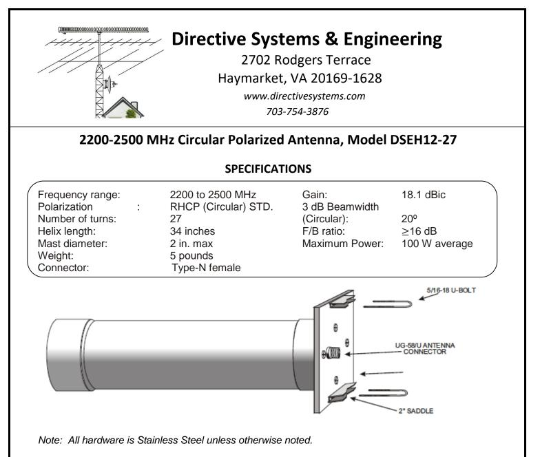
**Anti-Seize Compound** - Apply a small amount of the supplied Anti-Seize Compound to the aluminum joints and to the threads of the U-Bolts to prevent galling.
