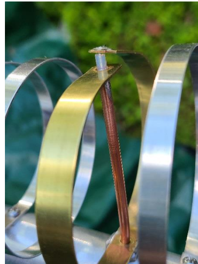
Soldered Driven Element
