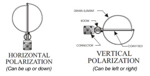
4) Attach the feed line, and tape it to the mast. The connector should be sealed with electronic grade RTV or equivalent.
