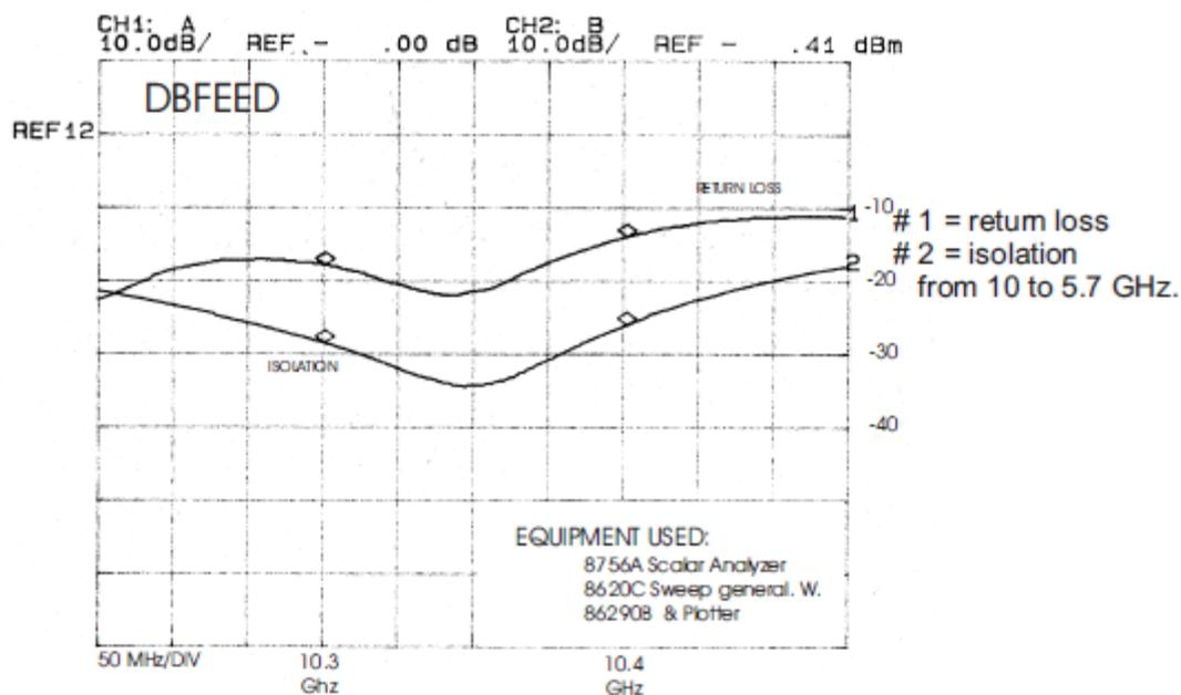
10 GHz isolation is quite critical and can be affected by what the feed "sees". It is always a good idea to check port to port isolation whenever you adjust the feed location on your parabolic reflector.
