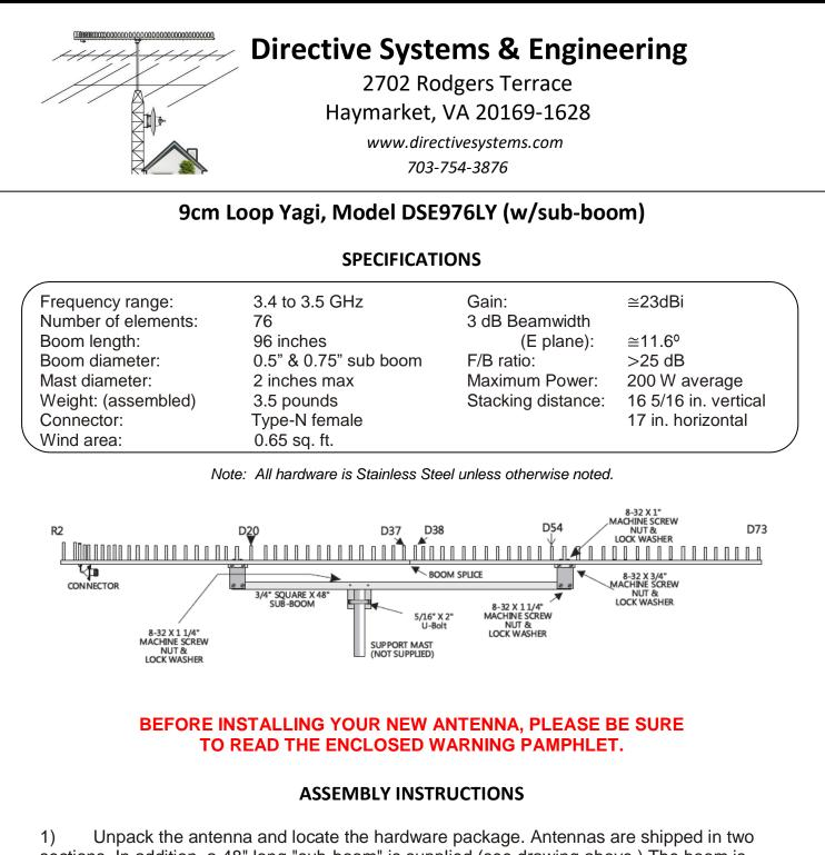
sections. In addition, a 48" long "sub-boom" is supplied (see drawing above.) The boom is broken between directors 37 & 38. Remove D38, D39 and D40 from the front boom section and slide the two boom pieces together. Use the alignment marks on the boom to correctly connect the boom pieces. Align the elements. Replace D3839 & D40 Note that D38-40 are all similar in size. Tighten the elements on the boom.
