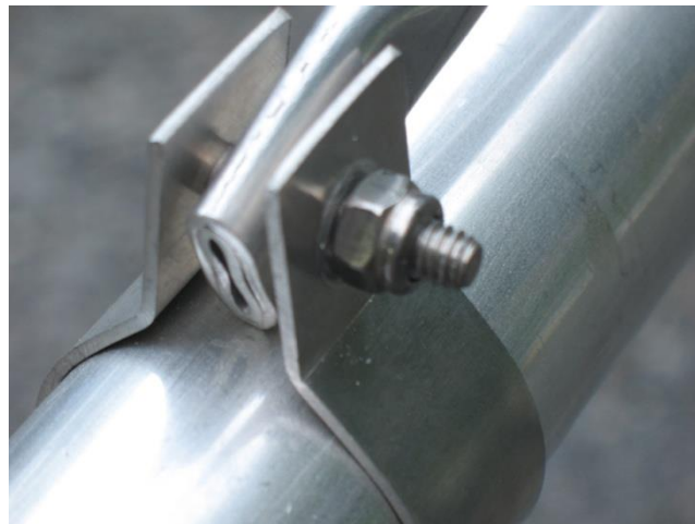
Photo 2: Boom Sag Strut attachment point
