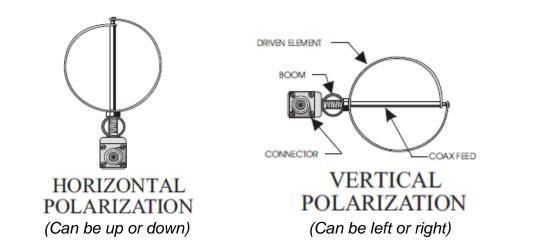
4) Attach the feed line, and tape it to the bottom of the boom. The connector should be sealed with electronic grade RTV or equivalent.
