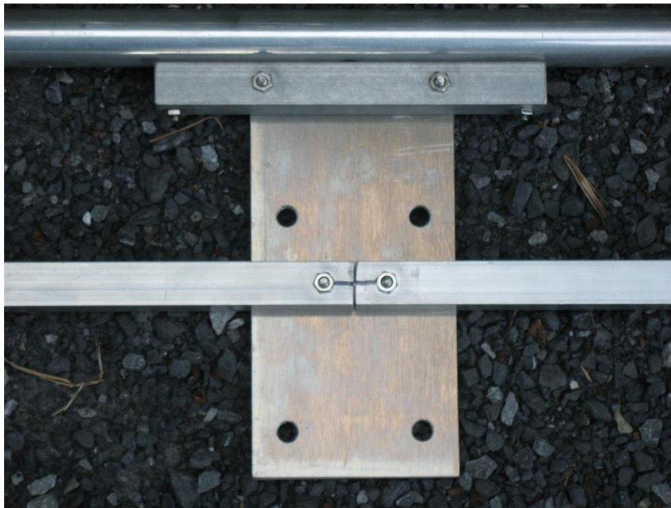
Photo 1: Boom to Mast Bracket and Plate
