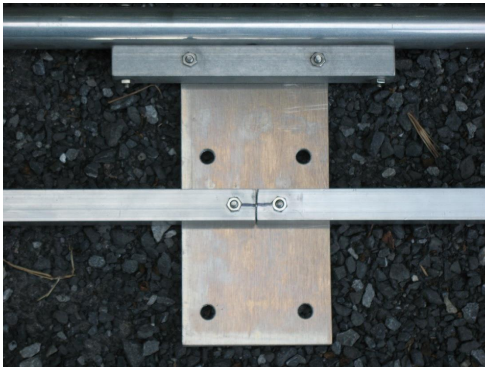
Photo 1: Boom to Mast Bracket and Plate
