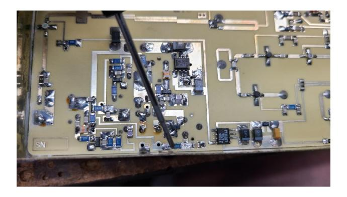
Next, remove the 2p2 chip cap that couples the oscillator into the first multiplier. I have my pointer on it.
