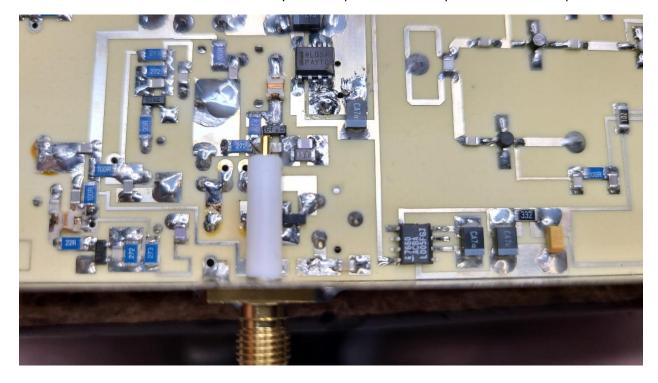
Next install the coupling cap from the SMA to the pad, my first attempt was with a nice 0603 chip cap. BAD mistake, the pix looks great but the small amount of flexing the case allows when I screwed on the LO cable promptly cracked the cap causing the output to drop WAY down.
